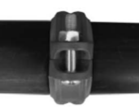
7 b. Assembly completed- Flexible Coupling For Flexible Coupling, two housings should be iron to iron connected. Gaskets can't be seen visually.
