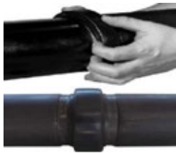
4.Alignment After aligning two pipe ends together, pull the gasket into position, centering between the grooves on each pipe. The gasket should not extend into the groove on either pipe.
